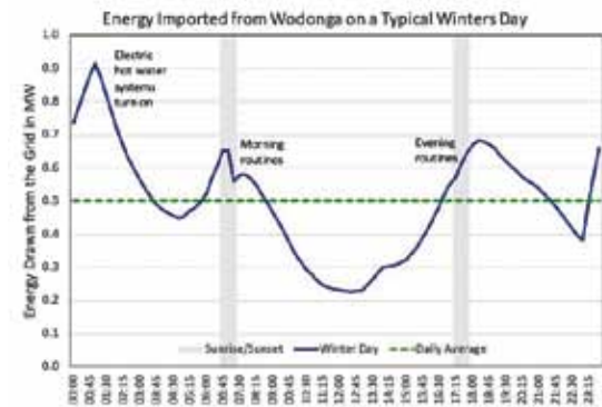
Total energy imports to the Yack township and surrounds on a typical winter's day. The Masterplan will identify how we can meet these needs. Credit: Mach 2 Consulting
