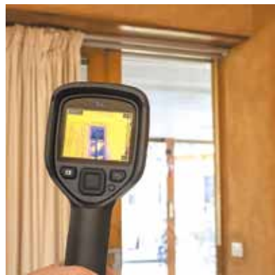
The IR camera showing what a difference good curtains can make. PC: Juliet Milbank
